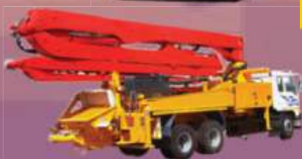
Boom Pump Concrete
